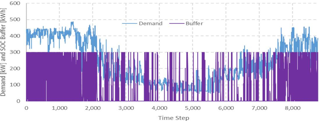
Figure 4: Demand and SOC of thermal buffer storage.
